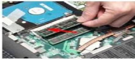
2. Press down to lock the DIMM module in place.
